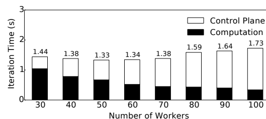
Figure 1: The control plane is a bottleneck in modern analytics workloads. Increasingly parallelizing logistic regression on 100GB of data with Spark 2.0’s MLlib reduces computation time (black bars) but control overhead outstrip these gains, increasing completion time.
