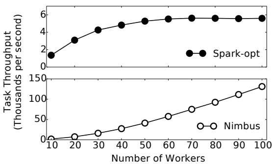
Figure 8: Task throughput of Nimbus and Spark as the number of workers increases. Spark saturates at about 6,000 tasks per second, while Nimbus grows to adapt to the number of tasks required for more parallelism. Note that the y-axis scale is different in the plots.
